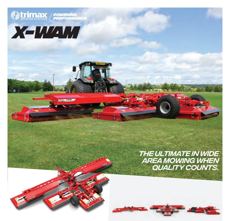
The X-WAM has superior contourfollowing abilities based on the unique combination of five individual floating decks on an articulated axis.
