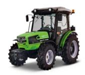
SDF 1000 Series Tier 3 Diesel Engine 4 Cyl/4000cc Turbocharged Intercooled Liquid/Oil Cooled Engine Speed Programming Individual Bosch Injector Pumps 95Hp @ 2200 rpm (2005/25/CE) Side Mounted Cabin Exhaust 70lt Fuel Capacity
