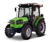
SDF 1000 Series Tier 3 Diesel Engine 3 Cyl/3000cc Turbocharged Liquid/Oil Cooled Individual Bosch Injector Pumps 62Hp @ 2200 rpm (2005/25/CE) Torque 244nm Side Mounted Cabin Exhaust 70lt Fuel Capacity
