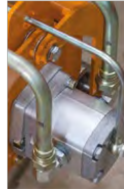
Direct Drive to reel shaft via hydraulic motor
