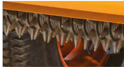
Studded roller for minimal surface disturbance and creating the seedbed ‘plant pots’
