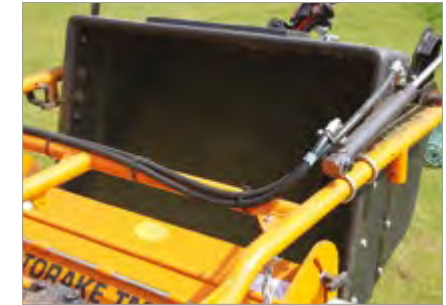
Large capacity collection box, shown with optional hydraulic tip kit
