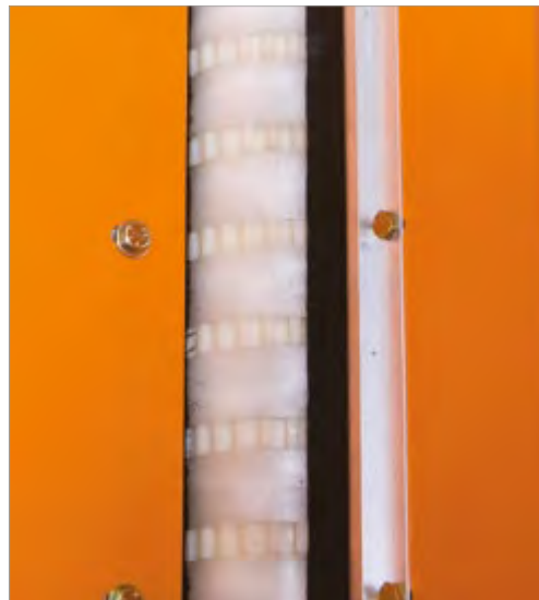
Grooved discharge roller – two discharge roller options for pure bent, rye grass/fescues
