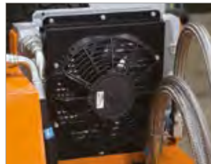
Integral heavy duty Oil cooler
