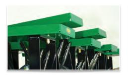
Each weight tray is capable of holding up to 150 pounds for better penetration in heavily compacted soil.
