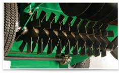
Durable cutting blades can be adjusted down to a depth of  $1\frac{1}{2}$ ".
