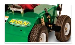
Self-propelled unit makes for easy operation and consistent ground speed.
