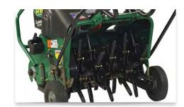
Redesigned tine assembly enables unit to be turned with tines in the ground, increasing productivity and reducing operator effort.
