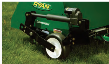
A variety of available lifting mechanisms allow you to easily lift and lower your aerating unit.
