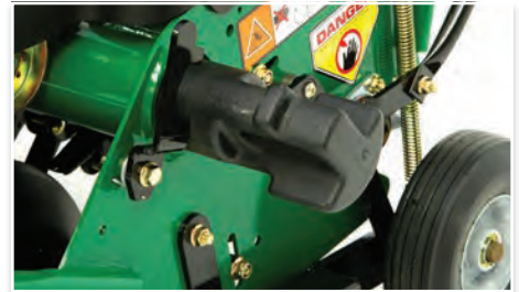
Weights are easily and conveniently removable for easier lifting and quicker, less strenuous transportation.
