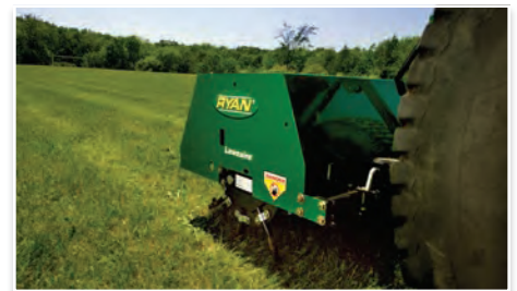
Reliable three-point hitch allows simple connection and is compatible with a wide variety of tractor models.
