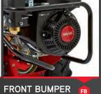
FRONT BUMPER Helps protect the front of the machine from damage.
