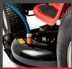
DECK WASH Helps maintain cutting deck in optimum condition by clearing away debris.
