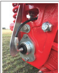
Central greasing allows for faster and easier maintenance.
