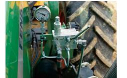
Adjustable hydro pneumatic **MU-SOFA** surface pressure relief for all front mounted implements to improve traction, to ensure the steering capability of the tractor, to optimise ground contour following, to dampen vibrations and protect the front-mounted implements.
