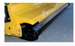
Bolt on wear plate inside the mulcher body with protection of the front cutting edge.
