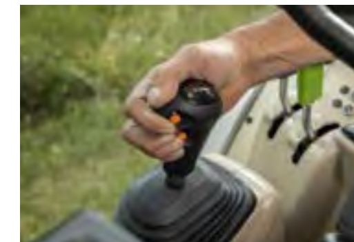
▲ New gear lever with bowden cable for smooth operation.
