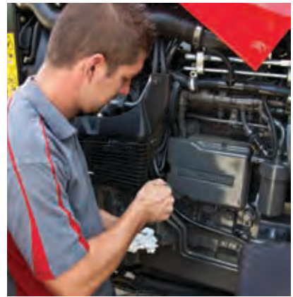
The waived bonnet and front axle design ensures comfortable access to the engine oil filters and oil dipstick
