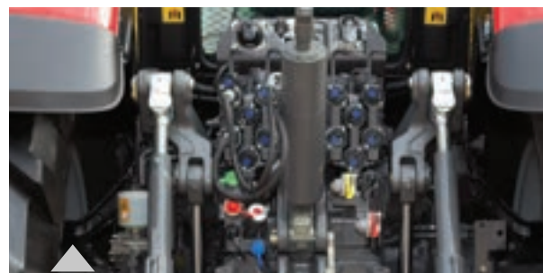
All rear couplers are equipped with an hydraulic decompressing system.
