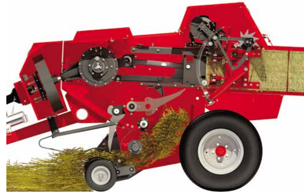
▲ Crop is moved directly from the pick-up into a pre-forming chamber.
