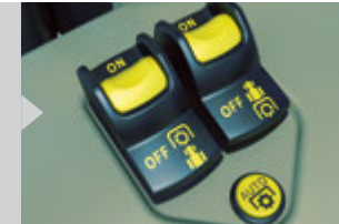
Command Centre PTO selector switches and Auto activation button.
