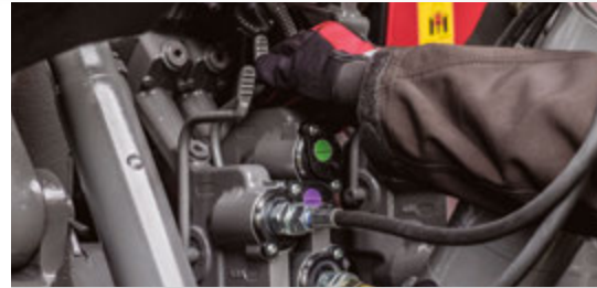
Conveniently located decompression levers
