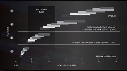
Dyna-6 offers six Dynashift changes in each range providing 24 forward and 24 reverse speeds, with an excellent overlap and a total of nine speeds in the Field Working range.
