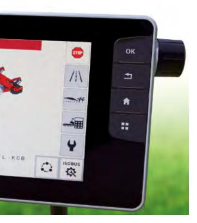
ISOBUS for total implement control – ISOBUS allows an implement manufacturer's control system to be displayed on the terminal screen, saving owners and operators time and money, with no need to install additional monitors in the cab. Simply plug the implement lead into the tractor's ISOBUS socket and the system automatically uploads the operating menus and displays on the screen. MF 6700 S ISOBUS applies to the AEF (Agricultural Industry Electronic Foundation) certification.
