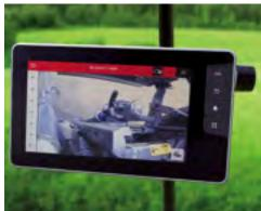
Video Mode — Pictures from an on-board camera can be displayed on the console screen, allowing operators to monitor complex implements or simply improve safety and efficiency when reversing.
