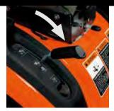
Release the lever to lower the deck
