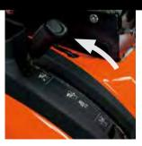
Pull the lever to lift the deck
