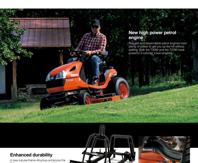
A new tubular-frame structure enhances the T Series already exceptional durability, rigidity, and strength. Even under tough terrain conditions—irregular lawn layouts, steep slopes, etc.—your T Series lawn tractor will continue to provide years of dependable service.
