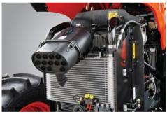
Turbocharged, Intercooled Engine
