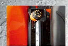
**9x3 Manual Transmission** Manual transmission models feature 9 Forward and 3 Reverse speeds delivering heavy duty performance. Second and Reverse gears are synchronized for efficient forward and reverse operations requiring frequent shifting.
