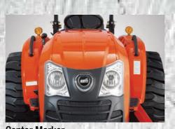
Center Marker The center ridge marker on the hood assists with maintaining straight rows.
