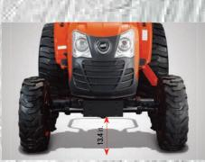
High Ground Clearance The maximum ground clearance of 13.4 in. makes usage on rocky or uneven terrain simpler.
