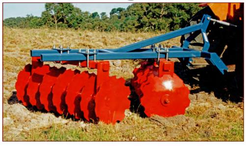
A robust, medium duty linkage offset disc plough designed for years of hard work with minimum maintenance. Australian made using high quality European Bellota discs.
