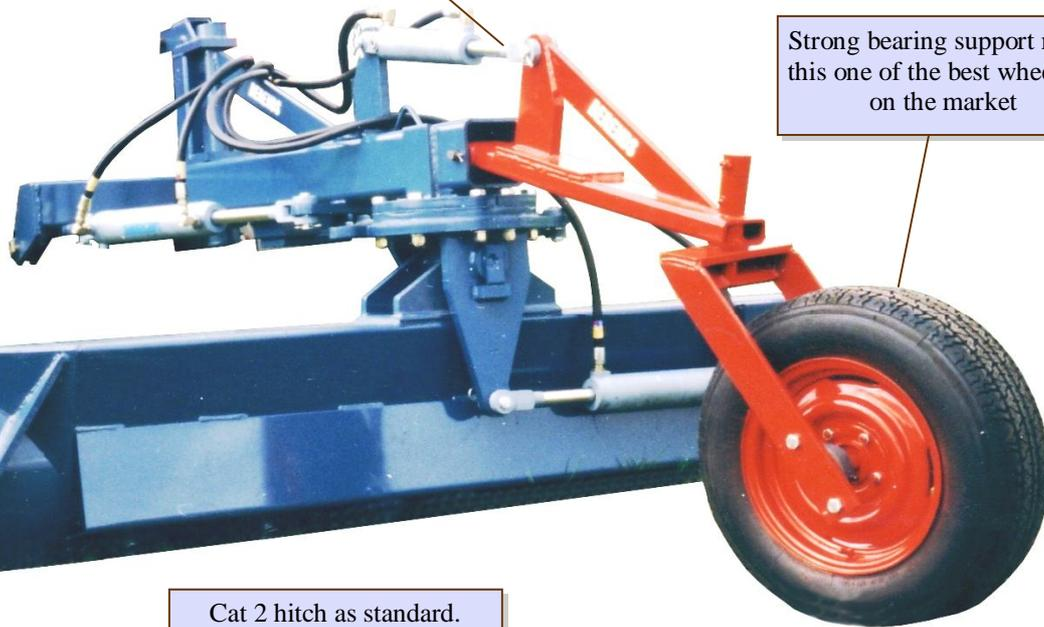
Hardened reversible cutting edge. Blade can be reversed for back blading work
