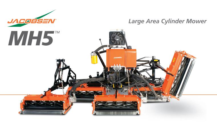
The Jacobsen MH5 tractor-mounted large area cylinder mower provides a unique, cost-effective alternative to traditional reel mowers. With the ability to mow or verticut, the MH5 turns your tractor into a versatile and efficient turf maintenance tool. Achieve excellent ground contour following and productivity with fully floating cutting units and a 3.43 m (135 in.) width-of-cut. Each cylinder is hydraulically driven with enough power and ruggedness to handle even the toughest conditions.
