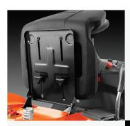
Adjustable driver seat Tool-free adjustment of seat position to quickly set a comfortable driving position.
