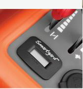
Automatic blade engagement The blades are engaged automatically, when you lower the cutting deck.
