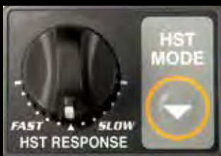
HST Response Control Dial and Mode Selection Button (only with HST Plus)
