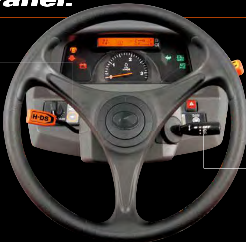
HST Response Control Dial and Mode Selection Button (only with HST Plus)
