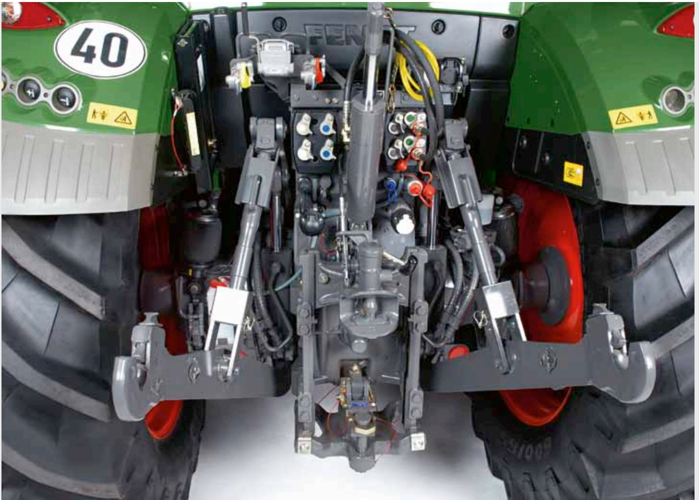
All the interfaces at the rear are arranged functionally and clearly. Signal socket, hydraulic top link, spool valves, unpressurised return, compressed air brake, pressure and control line power beyond, hydraulic trailer brake, 7-pin socket, lower link catch hooks, hitch, rear PTO 540, 540 E and 1000 rpm, bottom hitch, rigid drawbar and much more.
