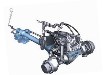
The secret of the exceptional climbing capability lies in the swinging power lift (V/F tractors) and the tractive point that lies in front of the rear axle. With increasing traction requirement, the weight that is transferred to the front axle is also increased. That enables high traction and climbing capability with minimum slip.
