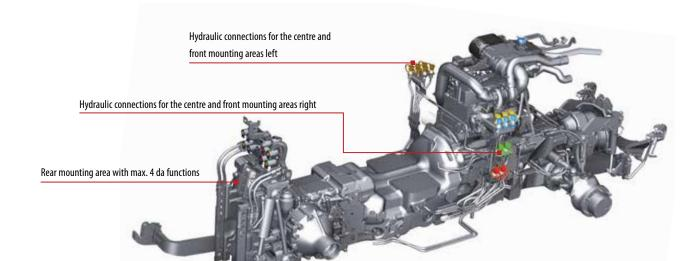
The electro-hydraulic rear linkage, with a maximum lift capacity of 2,715 daN (200 Vario V), guarantees that rear implements can be lifted over the full height without trouble. The standard-equipped shock load stabilising system counteracts vehicle bounce by actively lifting and lowering the power lift.
