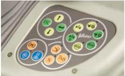
The 3rd and 5th control units can be actuated with the three On the dashboard, you can quickly and easily operate the multiple display, comfort engagement for 4WD, differential lock and front axle suspension as well as the Tractor Management System TMS.
