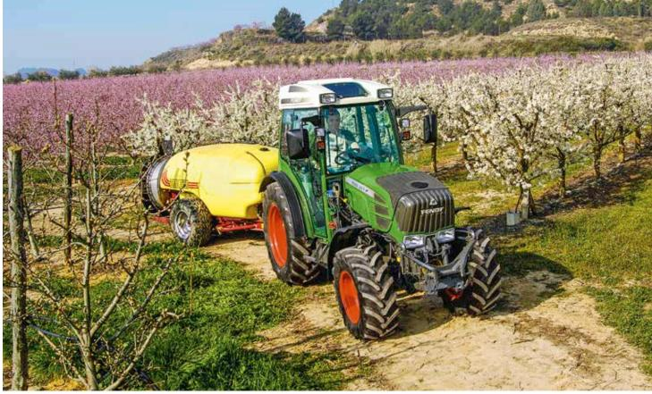
The self-levelling front axle suspension on the Fendt 200 Vario V/F/P specialty tractor guarantees maximum ride comfort, best driving safety and optimum traction. This provides considerable advantages on steep slopes, since all four wheels are in contact with the ground longer.
