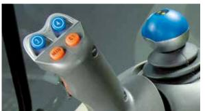
The armrest folds up to expose a rotary control that selects the button assignment for the multi-function joystick. The oil flow volume of the individual valves can be set with the rotary controls.
