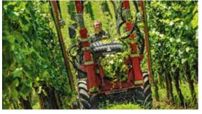
When cutting leaves, the suspension with anti-roll control dampens uneven ground reliability and sensibly with FSC. It ensures that working height and lateral tilt remain constant. Advantage for the driver: calm, relaxed work, because constant adjustments are not needed.
