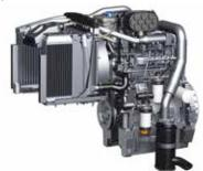
The efficient cooling system on the Fendt 200 Vario V/F/P has large intake areas. This results in less dirt in the radiator and optimised cooling performance, even during extreme operating conditions. The air filter features a cyclone precleaner, which guarantees a long filter life and less maintenance work. Despite the small installation space, it has a high air output.
