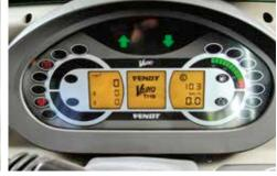
The clearly laid out instrument cluster has a speed display with cruise control, rpm display and multi-display.
