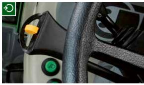
☐ With the reverser lever, changing directions is easily done with the left hand.
