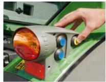
The Fendt 200 Vario has external controls for the linkage and rear PTO. Mount rear implements easily and save yourself unnecessary steps, for example, when filling the slurry tank.
