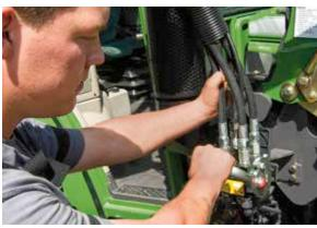
A multi-coupler connects all hydraulic and electric lines at once — even under pressure on the front loader side. The front loader can be quickly mounted and removed.
