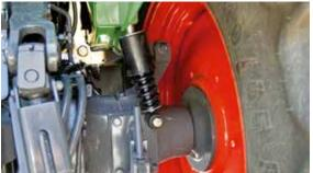
Thanks to the optional suspension, the Fendt 200 Vario cab is optimally supported on the rear axle. Shock loads and vibrations are absorbed by spring elements comprising shock absorbers and lateral stabilisers.
