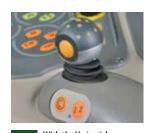
With the Variostick you can continuously accelerate the Fendt 200 Vario from a standstill to the desired speed, 0 – 40 km/h forwards and 0 – 25 km/h in reverse – without gear steps,
