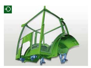
$\Box$  The Fendt 200 Vario can be fitted with cab suspension as an option. The cab rests on conical rubber bearings at the front, so that it is isolated from vibrations emanating from the tractor body. The helical spring shock absorber system at the rear of the cab reduces shock loads to a minimum.
