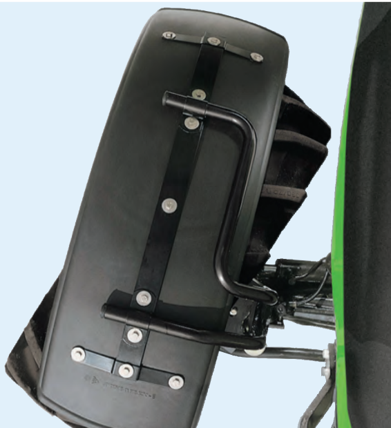
The swivel fenders fitted as standard reduce the tractor's turning circle.
