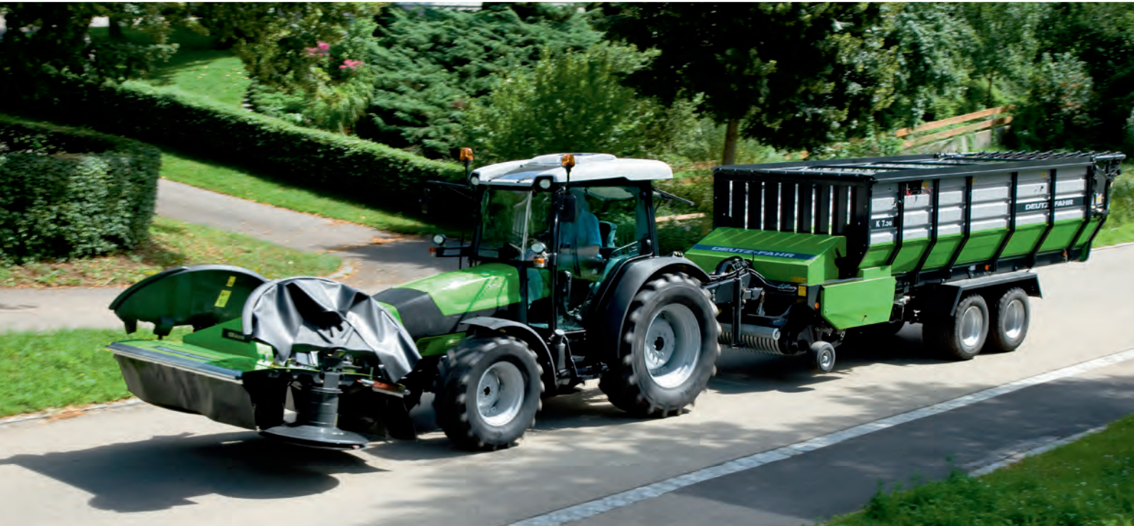
Low headroom is no problem for the Agroplus, thanks to its height of just 2.38 m (depending on model and tyres).
