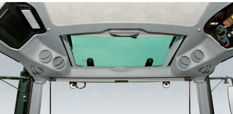
The front loader is totally visible through the high-visibility roof.
