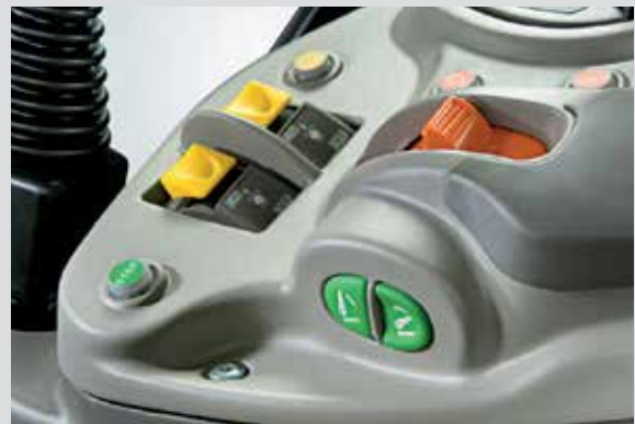
Easy to use headland up and down controls.
