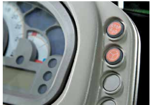
Stop and Go activation via push button.
