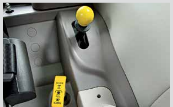
Easy mechanical PTO speed engagement.
