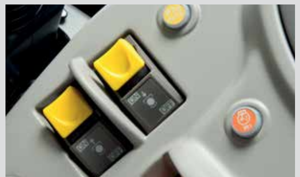
Electro-hydraulic switches to engage PTO.
