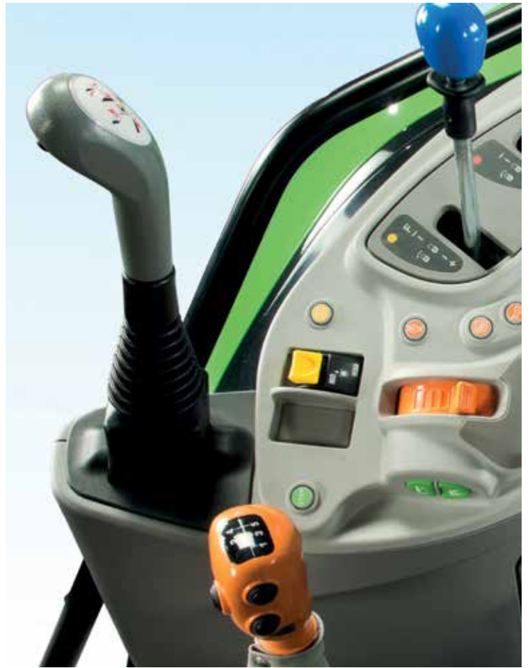
The loader control joystick integrates perfectly in the right-hand console.
