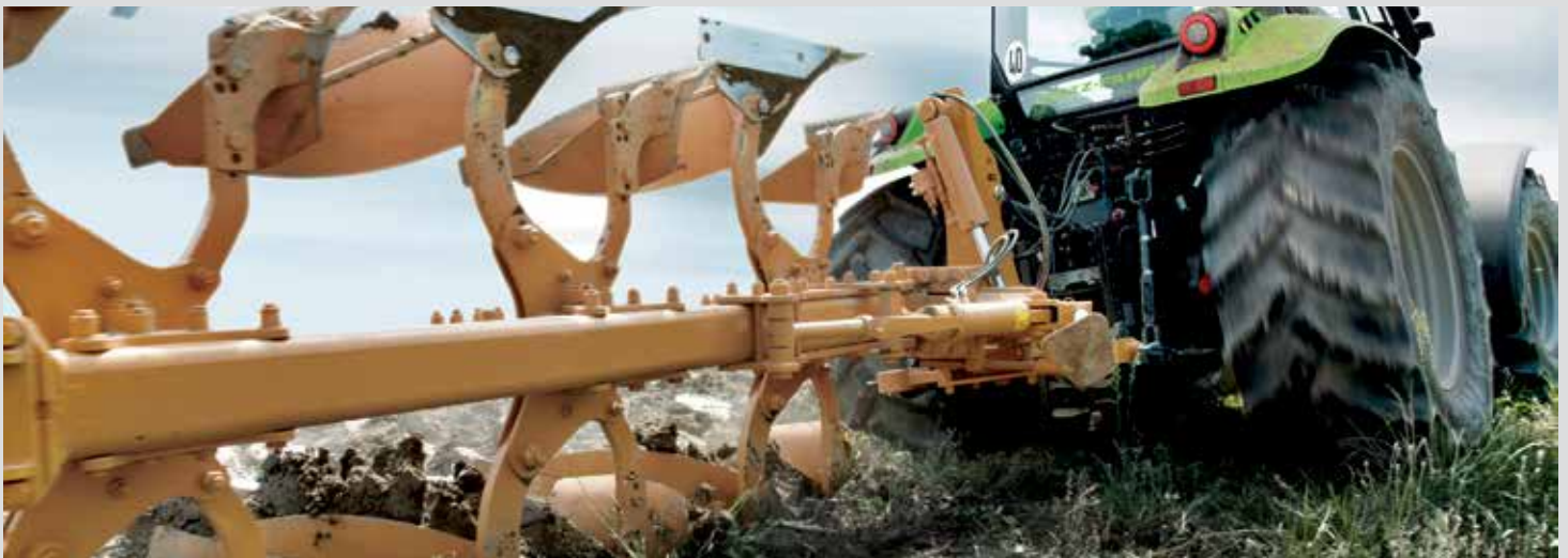
Heavy duty category 2 three point linkage.
