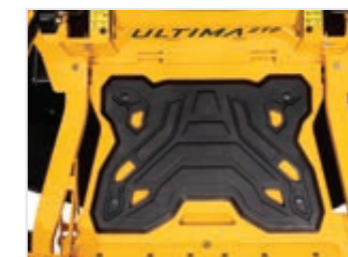
Rubber Anti-Vibration Footrest
