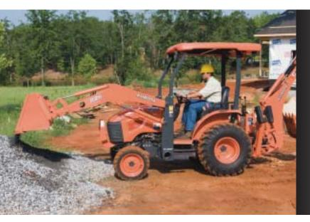
From the brace-less loader frame to the Skid Steer-type quick coupler, everything about this loader is designed to improve productivity. The B26's loader offers increased lifting capacity and a greater lifting height. It also has a host of features designed to make loader use easier, including a mechanical spill guard and a console-mounted joystick and armrest.
