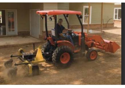
Built specifically for loader and backhoe applications, the B26 features an integrated main frame to ensure durability. Its 26HP engine provides high power and torque rise as well as low noise. And, a 3-point hitch greatly improves the B26's versatility.
