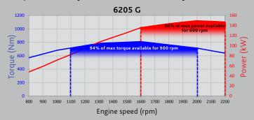
96% of maximum power available from 1600 rpm. Completely flat torque curve over an engine speed range of 900 rpm (from 1100 to 2000 rpm): almost maximum torque on tap across the entire operating range of the engine.
