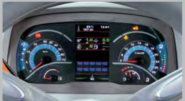
Cutting-edge instrument panel with new InfoCentre Pro : 5" LCD colour display and high resolution for a top-quality information concept customised by the user.
