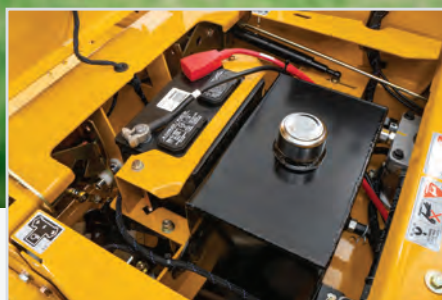
Heavy-Duty Hydraulics With 11 litre oil reservoir, oil cooler with fan & hot oil shuttle.
